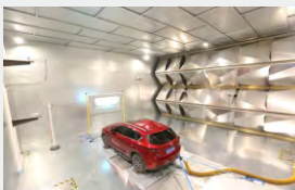
整车EMC/EMI 测功测试系统 Vehicle EMC/EMI dynamometer test system
