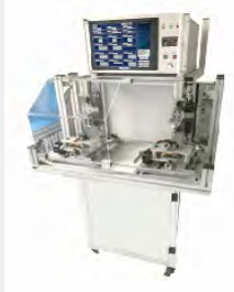
电机定点加载 综合测试装置 Integrated testing device for fixed point loading of motor
